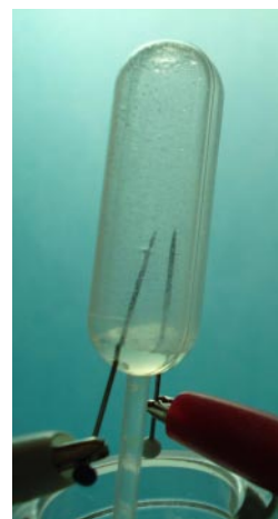
Figure 3. Electrolysis of water in a pipette head. (Most of the water is replaced by the mixture of its elements)
