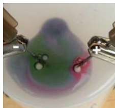
Figure 1. Drop electrolysis of a blue plant extract (left side is green, right side is red. After stirring it will be blue again).
